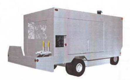
The 600 Series are truck or trailer mounted continuous flow jet engine starting units producing 250 to 270 PPM (depending on engine selection) at up to 40 psig start air pressure.
